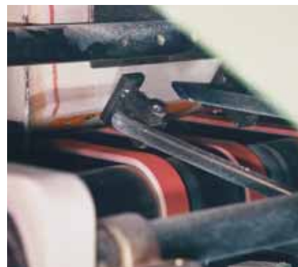
Accelerator belt for the discharge of stacked material in the manufacture of folded drinks cartons.
